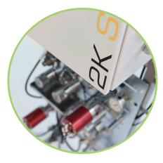
The WAGNER 2K Smart is an electronically controlled 2-K mixing and dosing system. Electronic mixing permanently guarantees the highest mixing accuracy and quick changes to the recipe. Another advantage of electronic mixing is that only the amount which is needed is mixed and therefore, waste is considerably reduced. The simple operability saves time and prevents operating errors.
